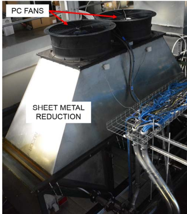
Figure 4-18. PC condenser cooling tower.
