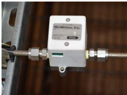
Figure 4-80. Bearing inlet volumetric flow meter.
