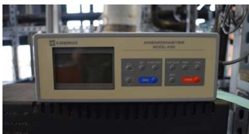
Figure 4-77. Kanomax anemomaster control module and LCD display.
