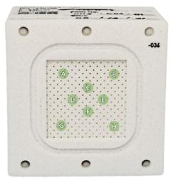
Figure 4-18: Impingement array height measurement locations
